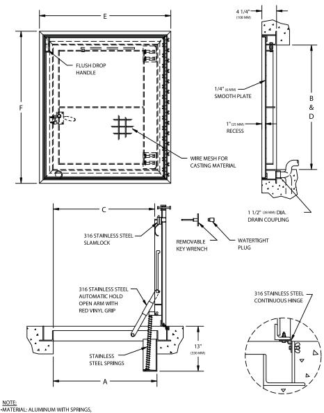
316 STAINLESS STEEL NUTS & BOLTS, SLAMLOCK, HINGES & HOLD OPEN ARM. -LOADING: 300 LBS. PER SQ. FOOT. (1464 KG. PER SQ. M)
